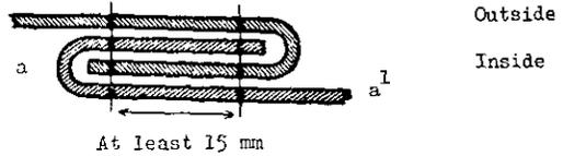
\*/ Threads visible from the inside shall be of a colour different from that of the threads visible from the outside and from that of the sheet.
